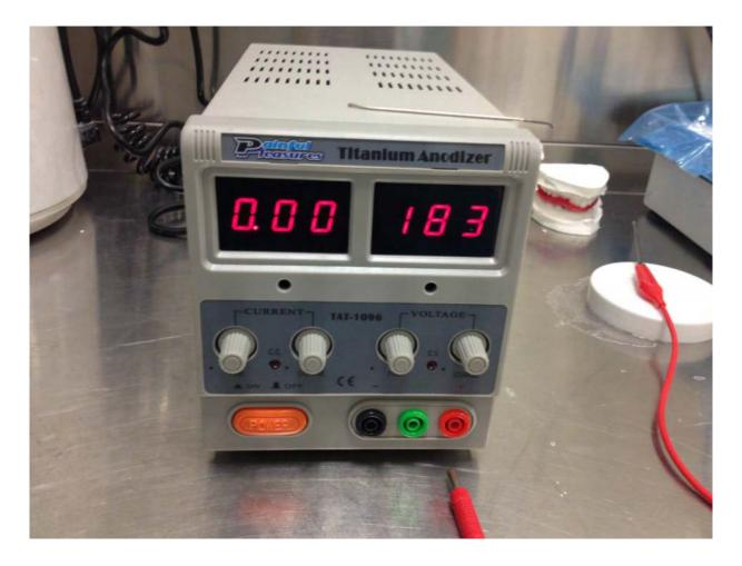
malfunctioning State: No load,Output Voltage>DC 100V Repairing step: First must cut off the power,it's very very important!!! 1) Take out this screw and take off the black panel, take out the screws on the shell and take offer the shell
