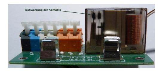
According data-sheet of the manufacturer this part survives min. 40,000 cycles, this means a life-span of 36 years with 5 copies per day on 220 days per year.
