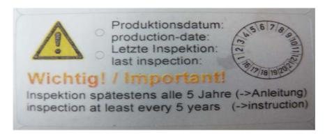
Since Jan. 2017 a label on the back of the machine shows the production-date. In case of maintenance please add a label with date (MM/YY). We can supply these labels upon request.
