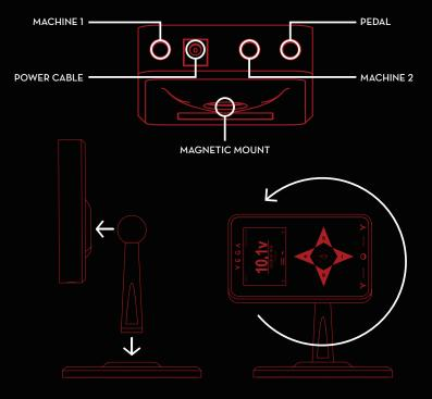
Your VEGA requires the use of the included magnetic mount for best defense against cross contamination. The preferred configuration is on the side of your cabinet or toolbox to free up your sterile work surface and allow for free motion of cords. The magnetic mounting can be adjusted 360°.
